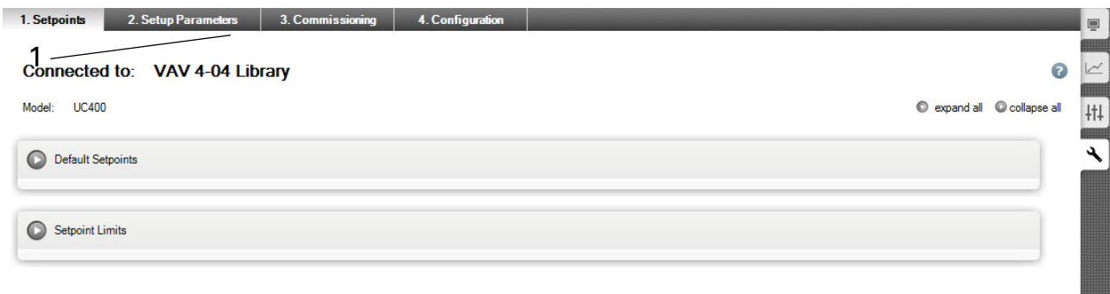
Figure 37. UC400 and UC210 configuration: navigate to setpoints using tabs
